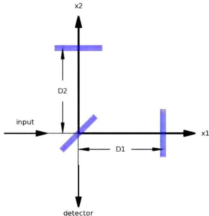
Measure voltage at detector as a function of time.
