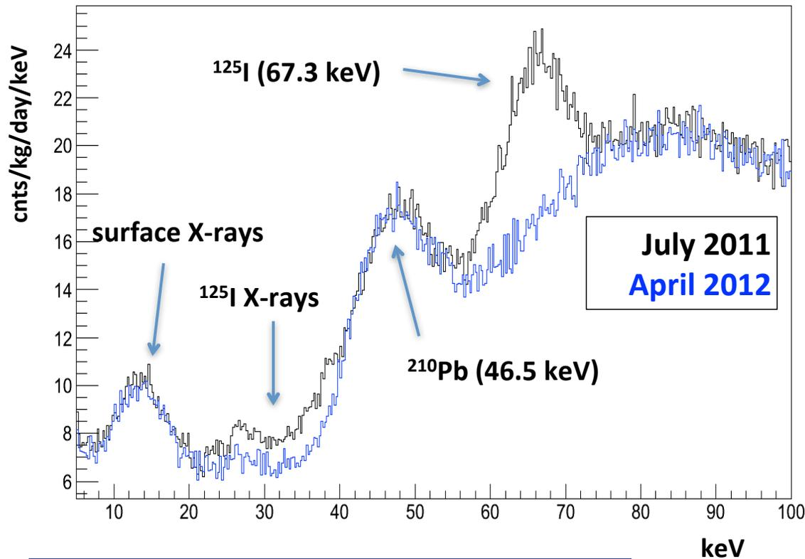
Cosmogenic lines verify our energy calibration; this is particularly useful for the prototype since we do not have an in-ice source.
