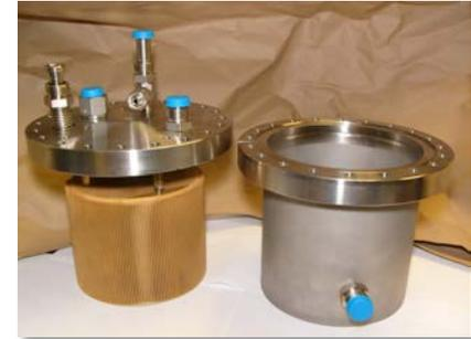
**Evaporator (left) and outer can (condenser)**
